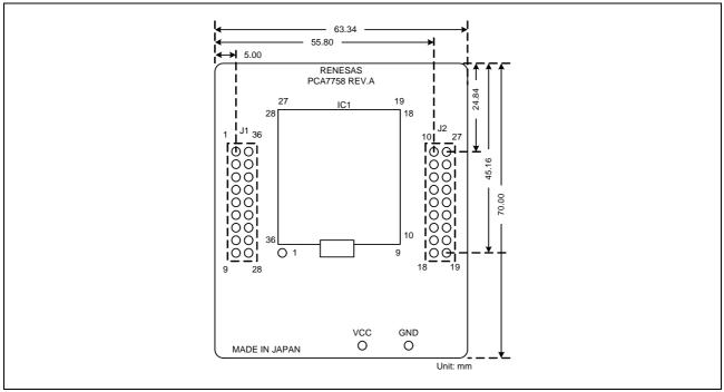
Figure 5 External dimensions of the PCA7758
